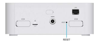
2. Press the SIM tool on the button for about five to six seconds, then your 5G Indoor Router will restart.
